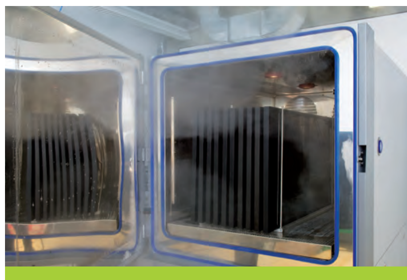
Sulfurcell’s climate chamber for accelerated module ageing
